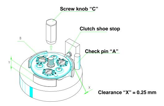
Place the clutch on the special tool code 143294 and block it using the screw knob "C". Position the clutch with one of the shoes blocked against the tool clutch shoe stop. Mount the main tool screw knob "C" and apply a constant torque of 8,5 Nm by using a dynamometric spanner tool with direct torque reading.
